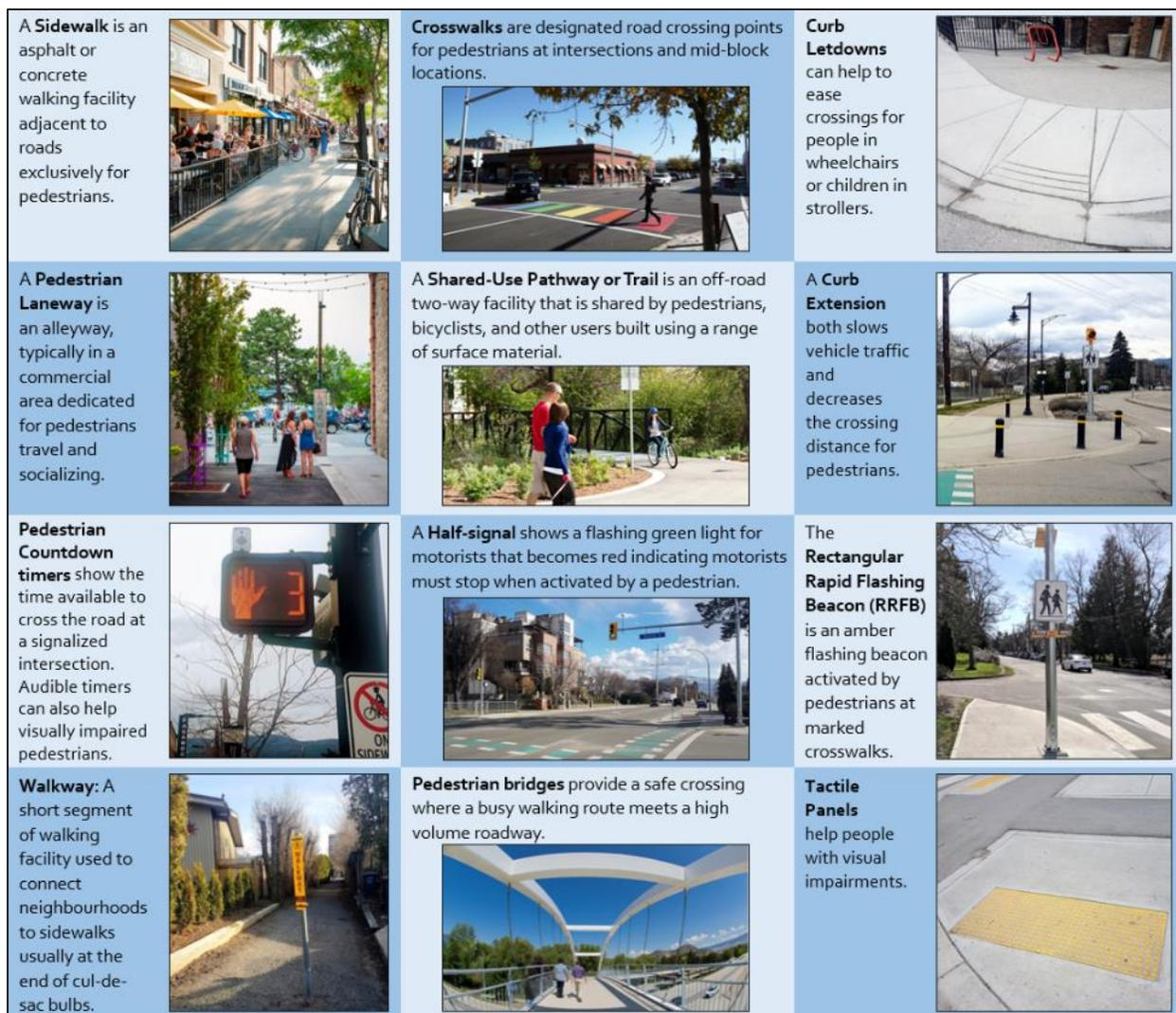
Figure 4a.7: Types of Pedestrian Infrastructure Installed Around Kelowna.
